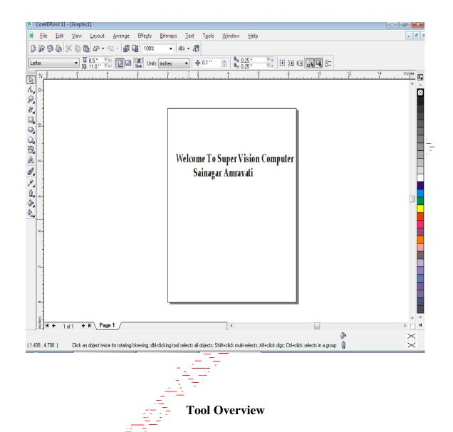
The Toolbox is located in the left portion of the window and contains all the drawing and editing tools necessary to create objects for an illustration. Tools containing a small triangle in the corner produce a Flyout. Flyouts contain additional tools or tool options and are explained below in the order they appear on the default screen. Flyouts are described following the Tool Overview.
