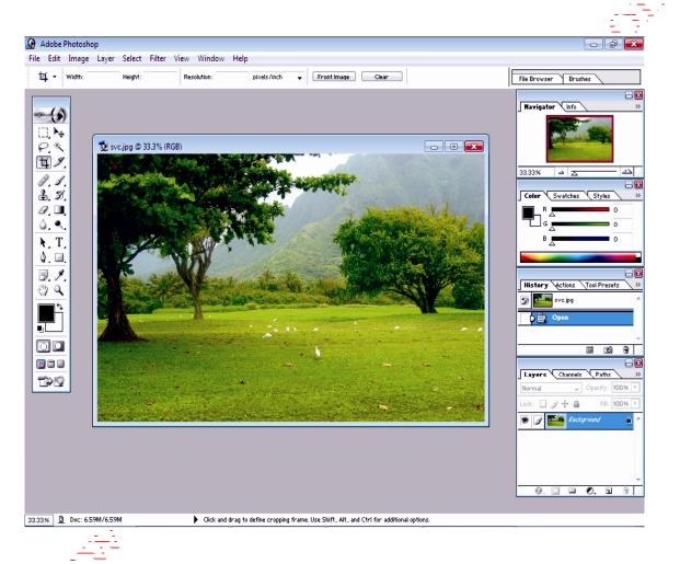
The first time you start the application, the toolbox appears on the left side of the screen. Some tools in the toolbox have options that appear in the context-sensitive tool options bar. These include the tools that let you use type, select, paint, draw, edit, move, annotate, and view images.
